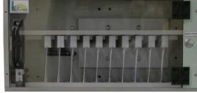
Torsion (twisting) - 10 cards on 1 test line This equipment tests the mechanical or electrical effects on a card submitted to repeated torsional stress. Test for contact cards, magstripe cards, RFID cards, dual cards, combi cards
